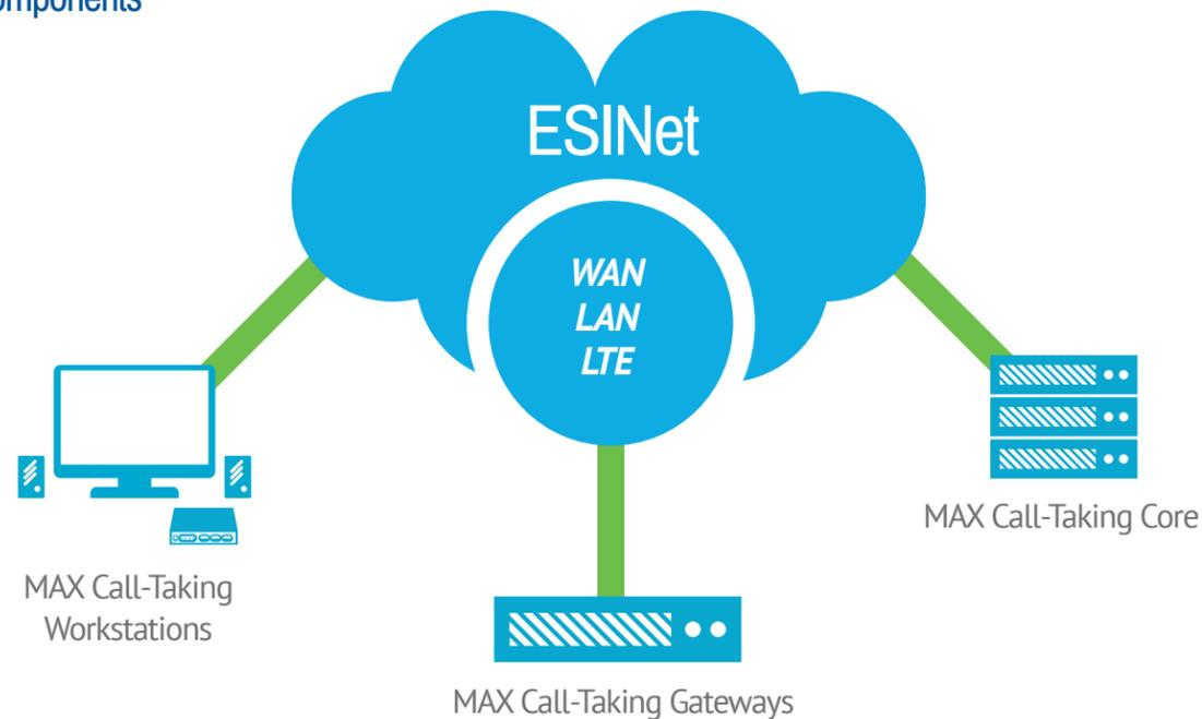
The main components of the MAX Call-Taking System are: the MAX Call-Taking Workstation, MAX Call-Taking Core, MAX Call-Taking Network Switches, and the MAX Call-Taking Telephony Gateways.
